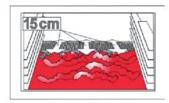
· CLOSE the LOWER VENT/DAMPER (as shown in the diagram below left)
