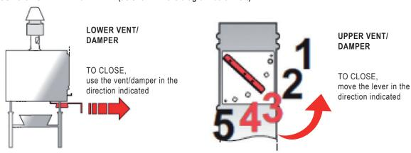
• Then, after 10 min., PLACE the UPPER VENT in position number 3, following instructions showed in the upper right diagram; these last two steps is the second cooking setting.
